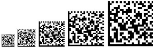
The area of the DMC should be not smaller than 1 cm<sup>2</sup> (10 × 10 mm) and not bigger than 4 cm<sup>2</sup> (20 × 20 mm). In exceptional cases, a one-off ruling can be made after consulting the responsible designer and SQE.
