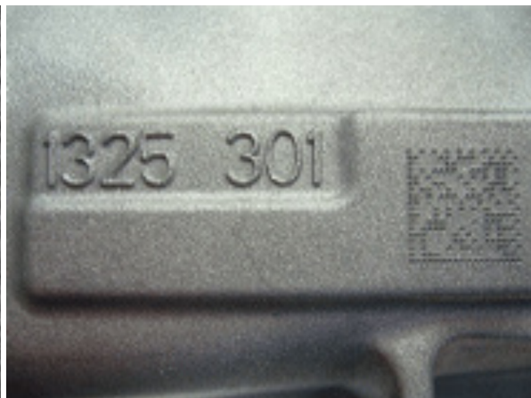
Direct data matrix markings on castings
